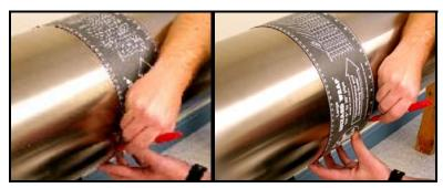
Figure 3-13: Marking Circumferential Lines on the Pipe
